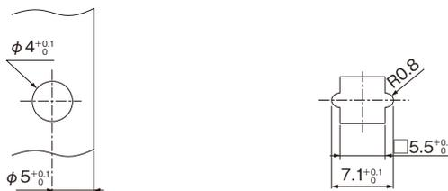
①基板側 / Board side : t1.6±0.15      ②シャシー側 / Chassis side : t0.8~2.3
